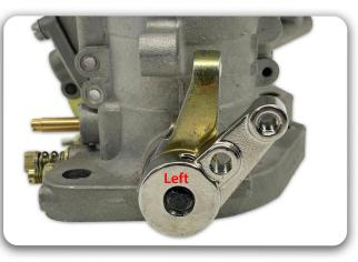
STEP 3 - Thread the "True Position" throttle arm onto the throttle shaft. Make sure not to overtighten as this can cause the throttle shaft to bind and not open or close smoothly.
