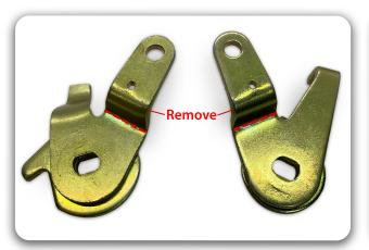
STEP 2 - For use on IDF Webers, the original throttle arms must be modified to allow the "True Position" throttle arms to be installed. Once modified, reinstall on the throttle shaft.
