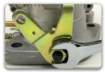
STEP 1 - Using an 11mm Wrench, remove the throttle shaft lock nut and throttle arm. Make note of which side the throttle arms are removed from.
