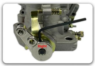
STEP 4 - Align the throttle arm so the set screws line up with the flattened sides of throttle shaft. Tighten the set screws securely using a 3/32" allen wrench.
