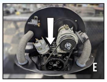
Remove any previously installed carburetor systems - Clean all gaskets surfaces. Remove center case nut and washer [E].
