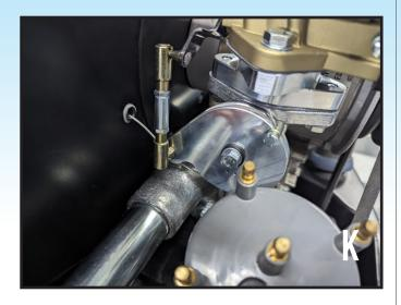
Tighten the barrel clamp onto the throttle cable, leaving a little bit of slack in the cable to avoid pulling the throttle open. Cut off the excess cable ½" past the barrel clamp [K].
