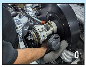
Feed the wires for the Sniper EFI kit underneath the alternator stand. Leave the temp sensor pigtail out of this bundle. Slide the intake tube into the boot for the 1-2 side end casting and position the intake manifold over the case stud [G].
