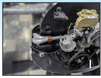
Install the 3-4 side end casting and boot/clamps on to the intake manifold. Go ahead and tighten the end castings and intake boot clamps at this time [I].
