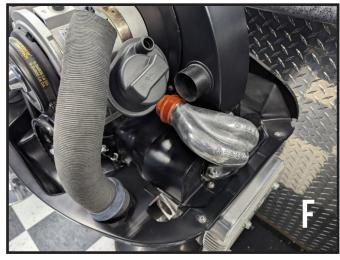
Install 1-2 side end casting with new provided boot and clamps. Leave it loose at this time [F].
