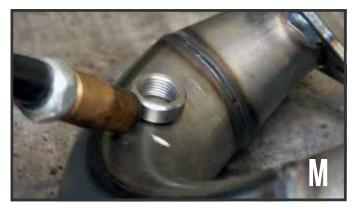
If a 4-into-1 header is being used, install the bung into the muffler head pipe a few inches away from the collector flange, preferably at somewhere between the 10 O'Clock and 2 O'Clock position [M].
