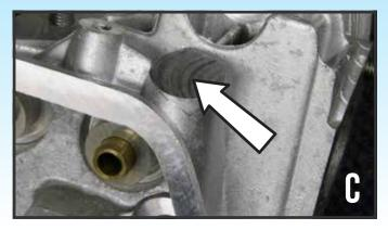
If you have an available boss cast into the cylinder head (New-Style CB 044's or Panchito 044's), you can use the boss [C].
