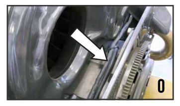
It is important that the wire harness is ran behind the fan shroud to help eliminate electrical noise interference. Make sure harness is zip-tied to the case so that it is not pulled into the fan while running [O].
