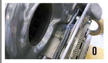
NOTE: It is important that the wire harness is ran behind the fan shroud to help eliminate electrical noise interference. Make sure harness is zip-tied to the case so that it is not pulled into the fan while running [O].
