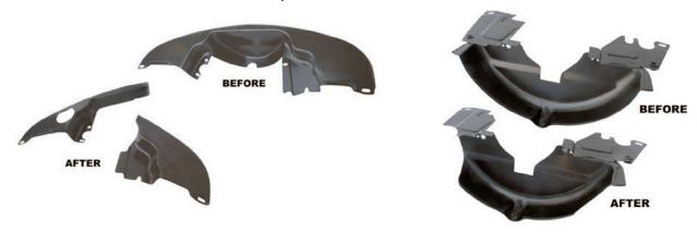
Here you can see some before and after pics of some Engine Sheet Metal that has been modified to run on a Turbo System.
