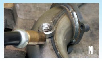
Turbo Applications: Weld the O2 sensor bung after the turbo. Please refer to the pictures to see the recommended placement of the O2 sensor [N].
